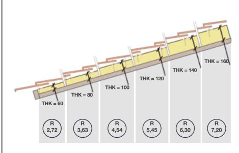
The wide range of thicknesses available in the **BORJATHERM** line, allows to get the needed thermal insulation for any type of house, enviroment or location, keeping the warm during winter and protecting from heat during hot season.
